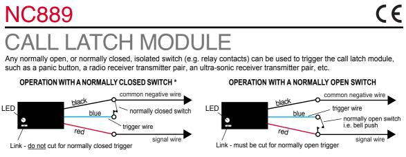
\* NOTE : If wiring the NC889 (with n/c switch) to a 10/20 Zone Call Contoller (NC910/NC920 series), connect the supplied pull-up resistor (8k2) at the call controller between the 'Zone' wiring terminal (Z1, Z2...Z20) and '+V' or '+V SW' terminal.
